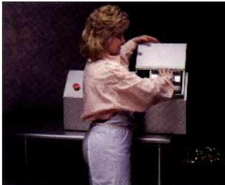
Place empty can in chamber.
